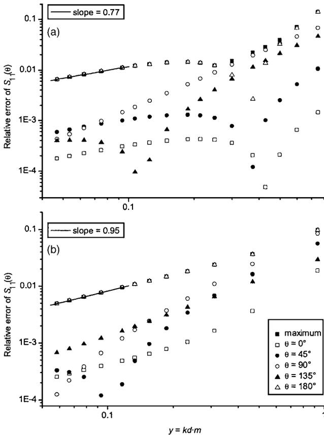
Fig. 3. Relative errors of  $S_{11}$  at different angles  $\theta$  and maximum over all  $\theta$  versus  $y$  for (a) the  $kD=8$  cube, (b) the cubical discretization of the  $kD=10$  sphere. A log-log scale is used. A linear fit of maximum over  $\theta$  errors is shown ( $m=1.5$ ).
